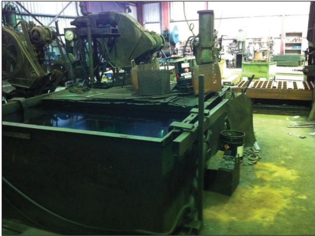
Plate 12 – Open tank filled with approximately 1,000L of tempering oil at Location 15, in the central portion of the Leaf Springs Shed
